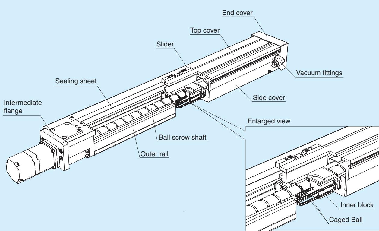
Structure of Clean-Room Actuator Model CSKR
