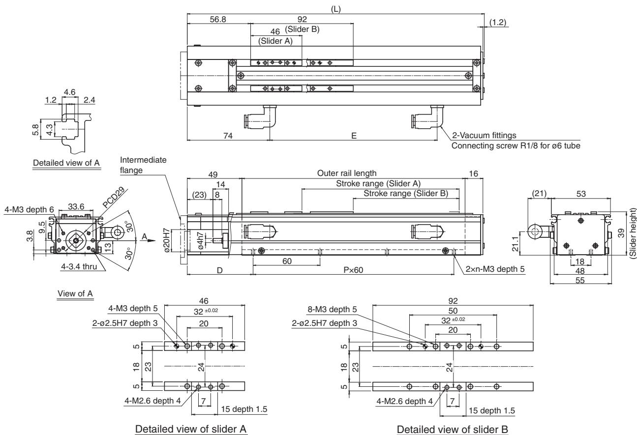
Note 1: The vacuum fittings can be mounted on either side.
