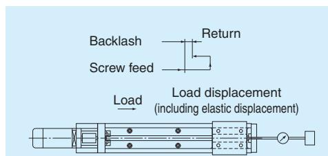
The accuracies of model CSKR are classified into normal grade (no symbol), high grade (H) and precision grade (P). The tables below show standards for all the accuracies.
