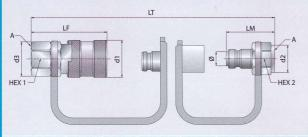
Note – Seal washer and connecting nipple included in HMV NIPPLE 1/4 are not represented on the drawing.
