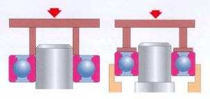
Special case of a long shaft for an assembly requiring a longitudinal adjustment of the bearing: it is preferable to use a mechanical coupling with a tapered seat joined to a bearing with a tapered bore.
