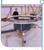
This device, especially developed for a wind turbine application, is capable of heating parts of up to 10 tonnes with an outside diameter of 4 metres to a temperature of 120°C in 60 minutes.
