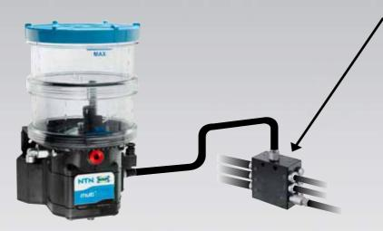
A «progressive» distributor includes at least three interdependent pistons. When the distributor receives the pressurised lubricant from the pump at the inlet, the piston is displaced and injects the volume of lubricant stored in the chamber from the other end. When it reaches its travel stop, the next piston is released and displaced. The lubricant received by the piston will be released during return travel, triggered by the travel stop of the previous piston.
