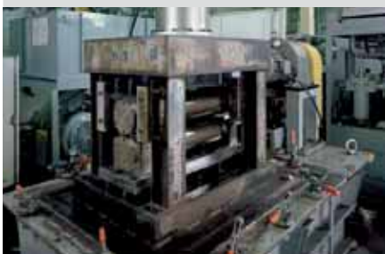
Test rig for bearings used in guide rolls of continuous casting machines
