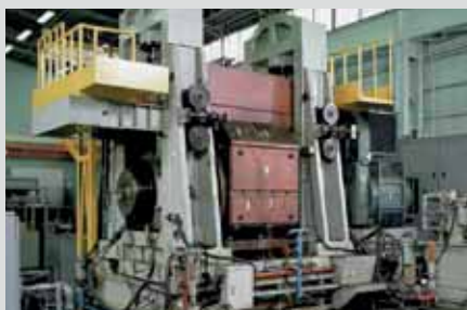
Test rig for bearings used in backup rolls of rolling mills
