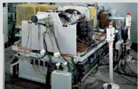
Test rig for bearings used in work rolls of rolling mills
