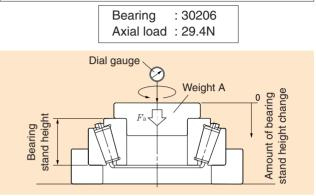
Fig. 7 Stand height stabilization test method
