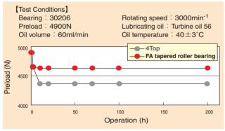
Fig. 6 Preload loss vs time test results
