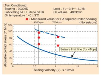
Fig. 5 Contact stress resistance test results
