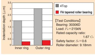
Fig. 9 Indentation depth measurement results
