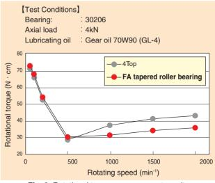
Fig. 3 Rotational torque measurement results
