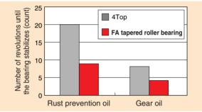
Fig. 8 Results of measuring number of revolutions until the bearing stabilizes
