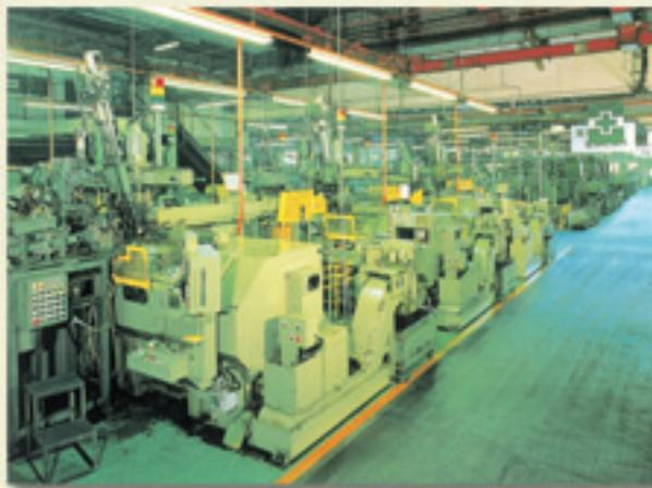
Turning process of outer rings
