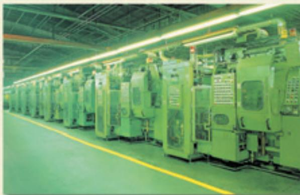
Grinding process of outer rings
