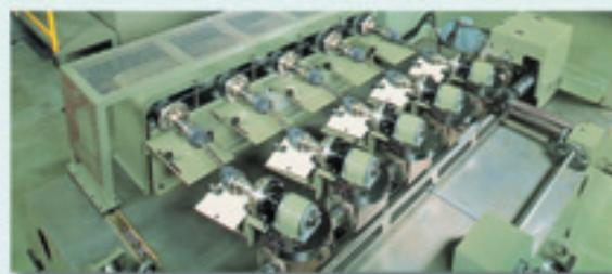
C.V. Joint boots durability testing machine
