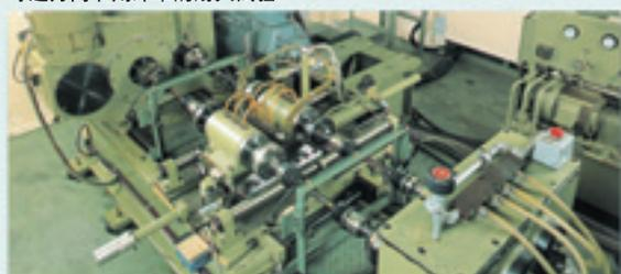
C.V. Joint high speed durability testing machine for propeller shaft
