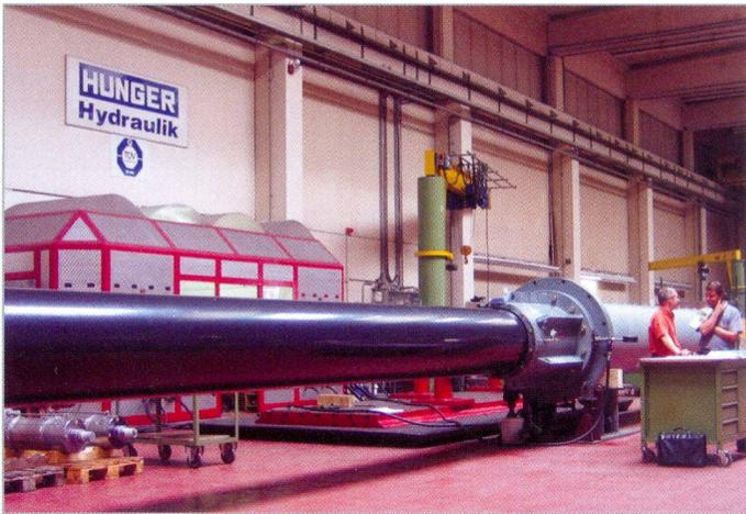
*Piston rods, axles, valves and rolls may have a severely reduced life when installed in aggressive environments (eg. hydromechanical equipment, mining industry, paper mill and printing industry). In addition to conventional surface protection systems such as hardening, nitriding, hard chrome plating and nickel plating, Hunger has developed a coating technology which significantly improves surface protection against chemical attack and mechanical wear and tear: Ceraplate.*
