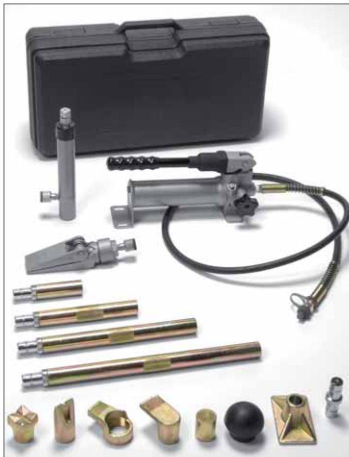
Set PPK 4 (art.nr. 7560804) incl. 4 t cylinder, 100 mm stroke, in portable transport case
